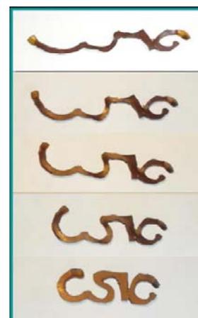
Shape recovering of carboxylated nitrile rubber (XNBR) after being deformed to transitory shape and following a temperature increase over ionic transition temperature.
