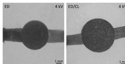
Micrograph of dielectric elastomer showing the response at 4 kV without LC (left) and with LC (right).
