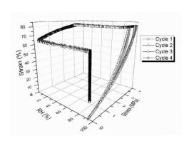
Humidity-mechanical cycles. 2D stress-strain cycles and 3D stress-strain-temperature cycles diagrams, at the top and at the bottom respectively.
